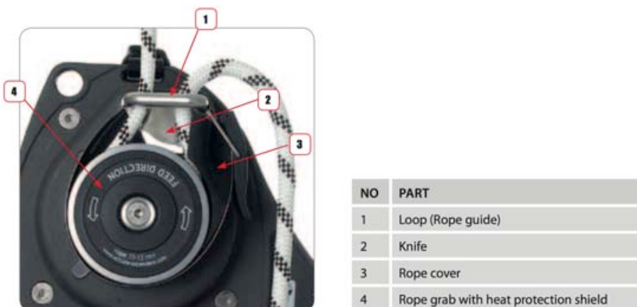
Figure 1. ActSafe ACC powered ascender drive system nomenclature of parts.
